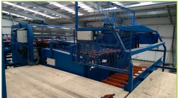
One of the two layer crosscut- & stacking lines (line "B") at James
