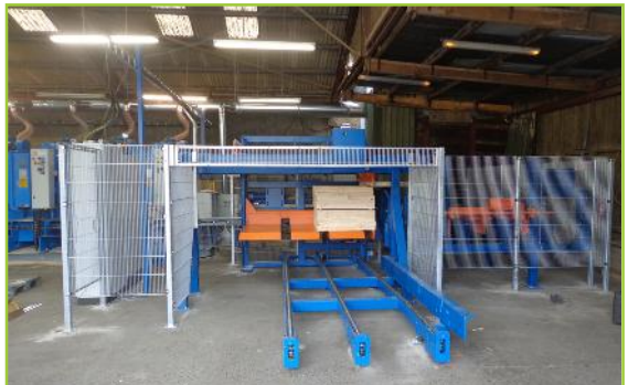
At Woodfab Timber Ltd.: the infeed for the resaw-line for short products
