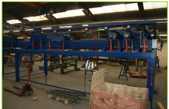
View of a total of 6 stick magazines for one of the stacking machines for Murray Timber's new line.
